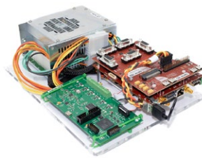
The Tulipp Starter Kit with Lynsyn PDM on a PC/104 carrier board.
