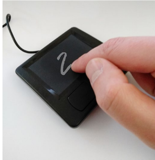
AifES demonstrator for handwriting recognition. Numbers written by hand on the PS/2 touchpad are identified and output by the microcontroller.
